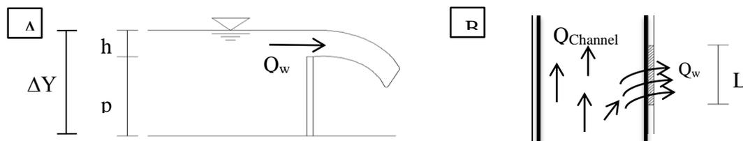
Figure 4. Weir schematics: A: Lateral view of the weir; B: Top view of the weir.
