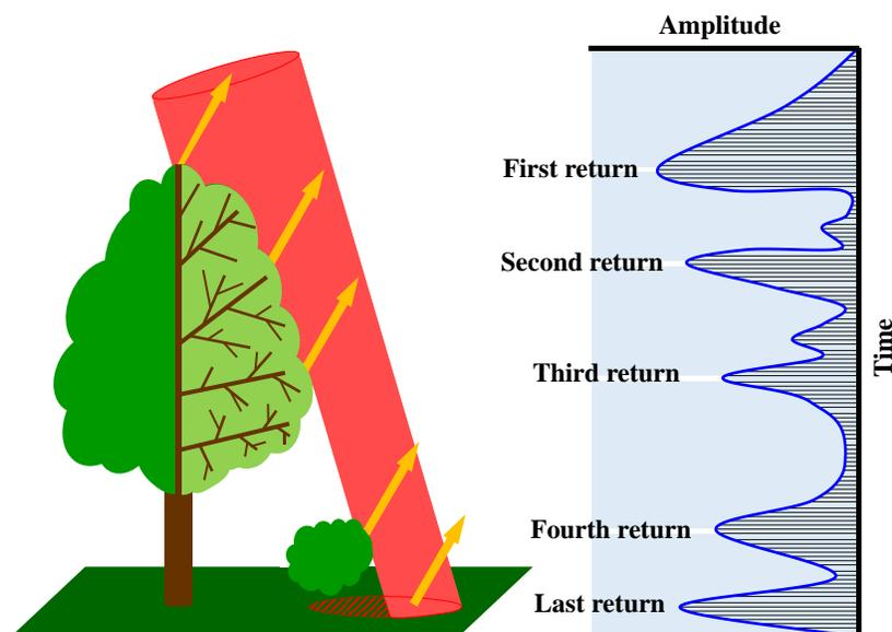
Figure 1. Multiple echoes and digitized waveform
