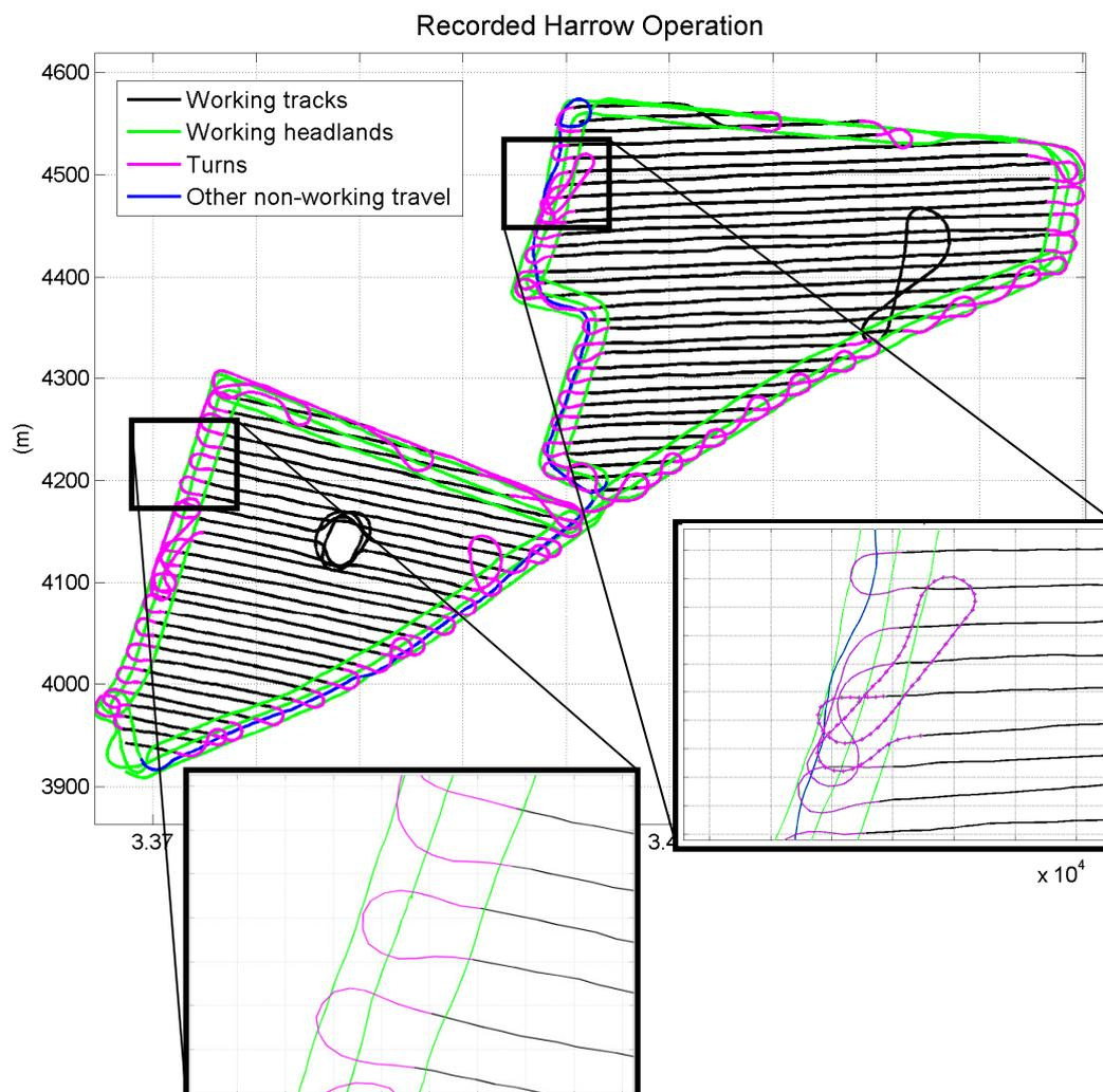
Figure 2 - Plot of the segmented recorded path of the tractor. The left insert shows how turns are defined as starting at the innermost headland pass. The dotted pink path in the right insert is an example of a turn outlier which should not be included in the turn model fitting.
