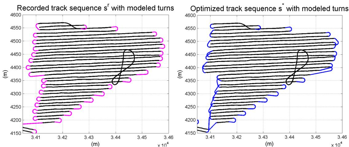
Figure 4 – The left plot shows the recorded sequence with modeled turns. The right plot shows the optimized sequence with modeled turns.
