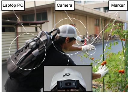
Figure 1. Parts of Hand Framing Camera
