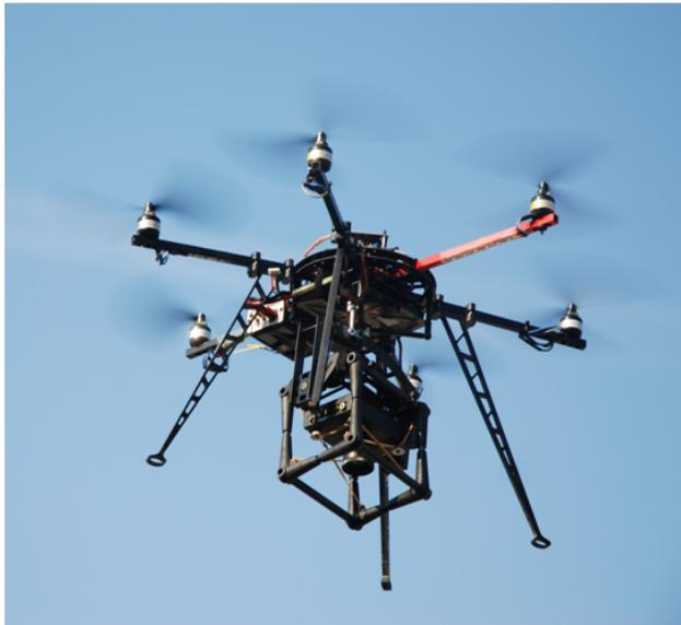
Figure 1. Mikrokopter Hexa with custom-built camera mount.
