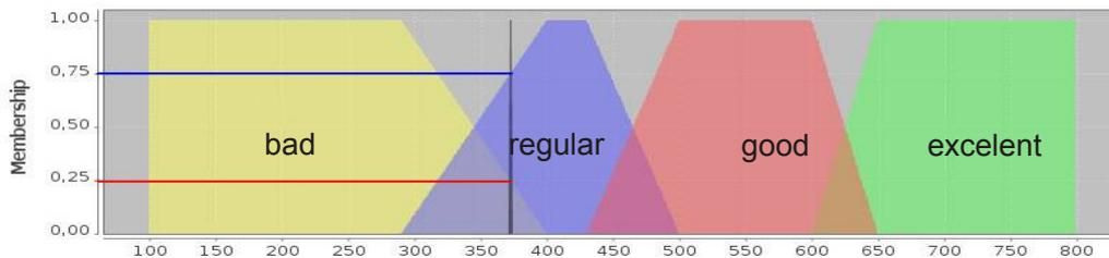
**Fig. 3.** Fuzzification process.
