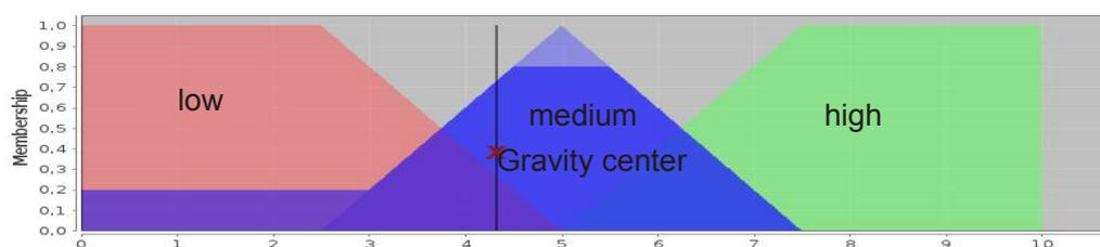
**Fig. 4.** The defuzzification Process.
