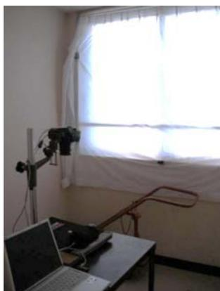
Figure 2. Scheme of color acquisition system under natural lighting condition.
