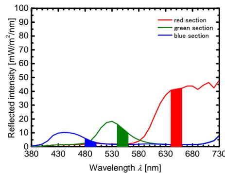
Figure 5. Reflected intensities of illuminating light on red, green, and blue sections of standard color chart and wavelength characterizing natural lighting illumination.
