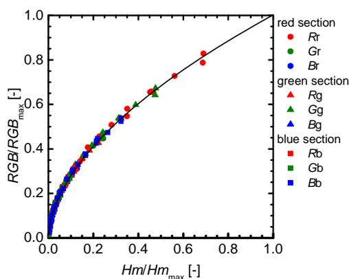
Figure 4. Normalized relationship between  $Hm$  on RGB values of sample objects under white lighting.
