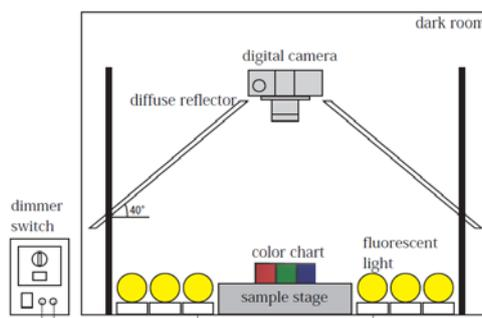
Figure 1. Scheme of standard color acquisition system.
