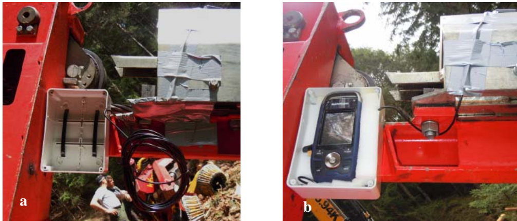
Figure 1. Installation of GNSS device on carriage.
