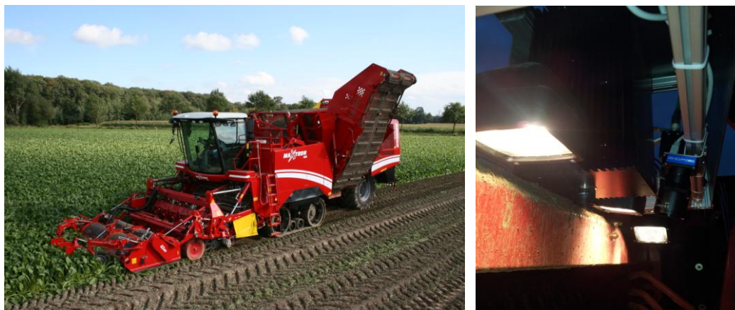
Figure 2. Grimme Maxtron 620 sugar beet harvester (left), developed HIS system implementation above the conveyor belt on the harvester machine (right)
