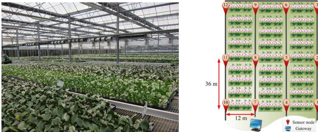
Figure 2. Real world testing: (a) The practical experimental environment; (b) The layout of sensor nodes and a gateway
