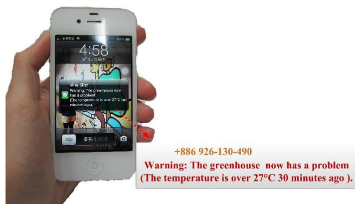
Figure 4. A warning message sent by the alerting function
