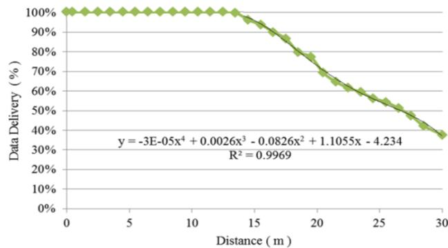
Fig.5 The regression of the successful rate of data delivery and distance between the active and failed gateway
