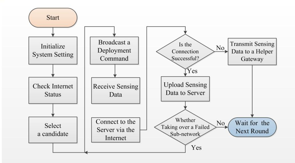
Fig.4 The program procedure of the gateway with the automatic data backup mechanism
