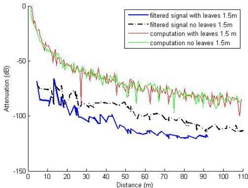
Figure 3. RSSI computations and measurements for transmitter and receiver height equal to  $h=1.5$  m.
