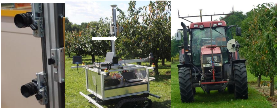
Figure 2: Arrangement of the cameras on the University of Hohenheim-designed autonomous platform (left) and the laser on the tractor in 2012.
