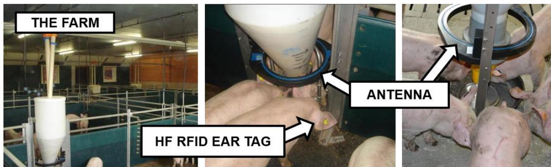
Figure 2: Trough with RFID HF antenna
