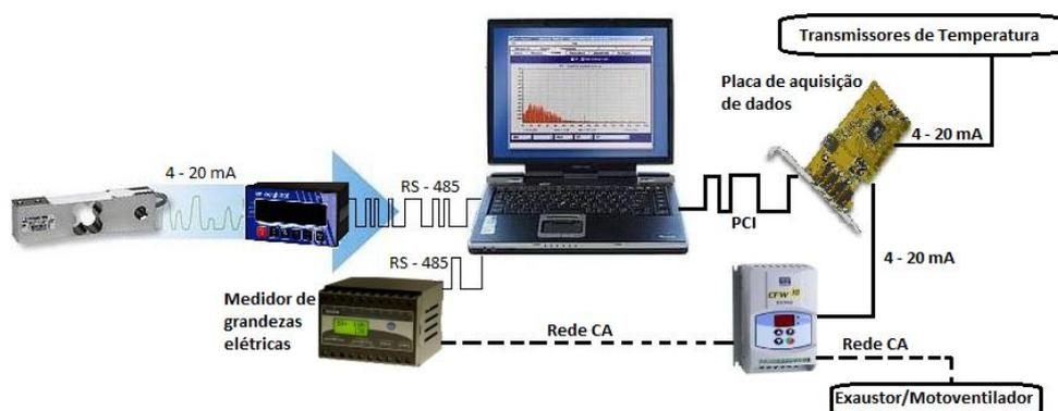
Figure 1. Scheme of the data acquisition process.
