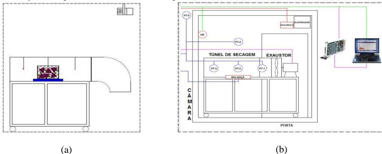
Figure 2. (a) Schematic structure forced-air drying, (b) Schematic instrumentation system.
